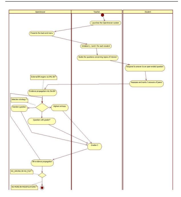
Figure 2. The Activity Diagram of the assessment process.
